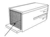
Screen is 7x7" galvanized hardware cloth (19 ga./  $\frac{1}{2}$  holes). Fasten with 6 – 16 ga.  $\frac{1}{2}$ 6" x 2" glue collated staples (2 on each side and 2 at top of screen).
